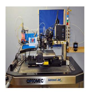
"The Aerosol Jet offers us the ability to develop future products that we could never have thought of producing before. We can lay down traces as small as 8 microns [0.008 millimeters]. That means we can put many more recording elements on the same amount of space as we do now. It's a game-changer for us."
